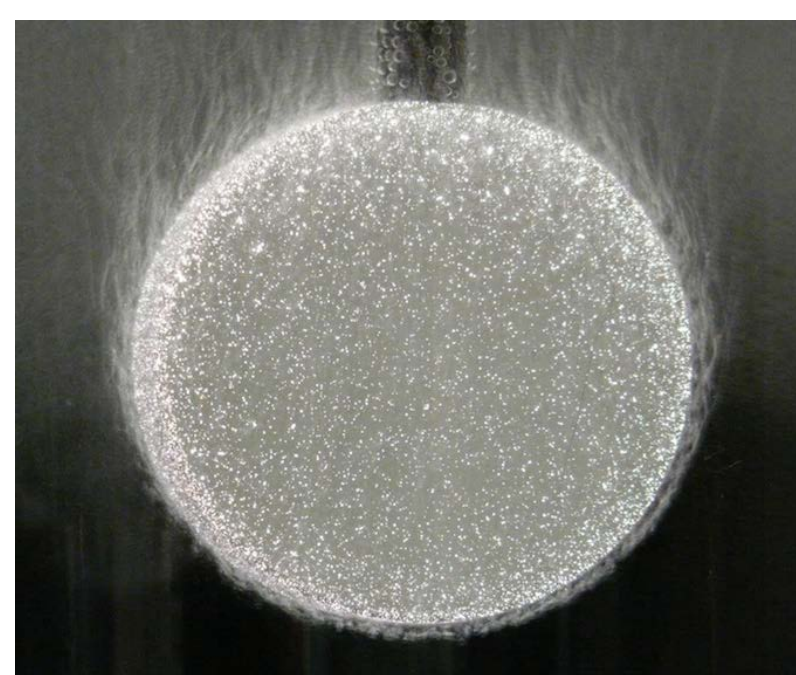
Figure 1: Surface plasma interacting with metal sample in electrolyte baths [2].
